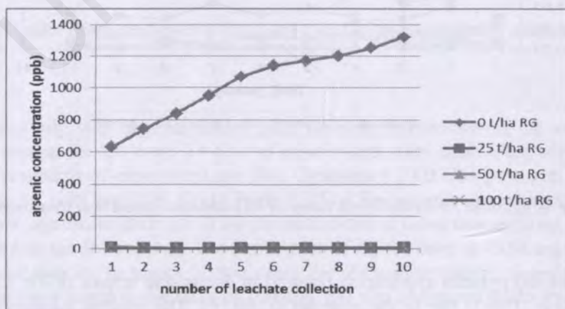
Figure 7: Arsenic concentration in each of the leachate collection (50 ml) up to one pore volume for each treatment.
