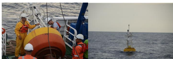
(Left) Deployment of METOcean buoy. (Right) METOcean buoy mooring in the South China Sea.
