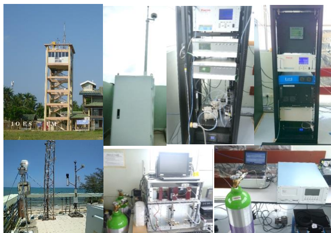
(Left to right) GAW observation tower; optical particle counter; O_3 , SO_2 , NO , NO_2 sensors; central logger, N_2O , CO_2 , CH_4 , H_2O sensors; CO sensor; micro-Dirac sensor; sonic anemometer.
